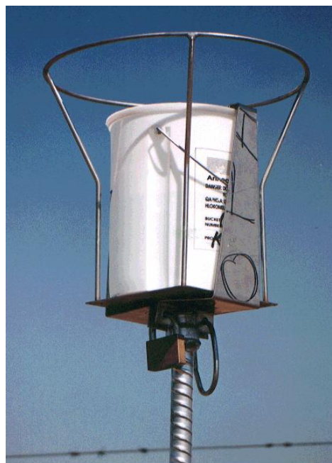
Figure 1: Single bucket monitoring unit, showing a sampling bucket with bird ring and security clamp.
